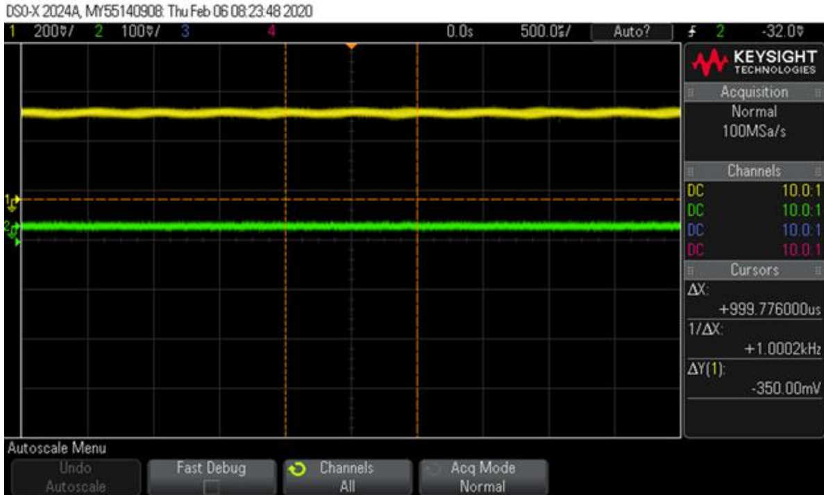
Figure 5.6.14 Full Wave Rectifier Testing with smoothing capacitor 10K ohms load 20uF smoothing cap
