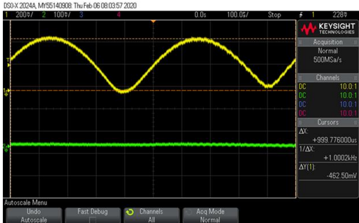
Figure 5.6.11 Full Wave Rectifier Testing Output 4 1000 ohms load
