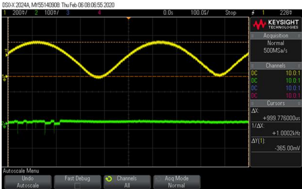
Figure 5.6.9 Full Wave Rectifier Testing Output 2 330 ohms load
